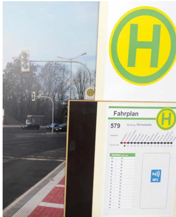
Figure 39: IoT Device Bus Line Information with NFC
