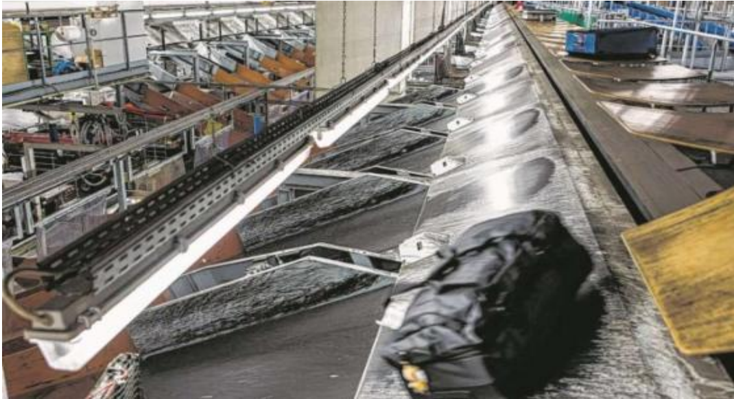
FIGURE 21: Circular sorter system with baggage chute at Hamburg Airport
