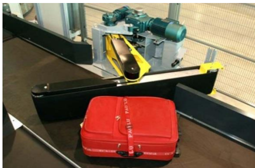
FIGURE 26: Swing-panel sorter (a; b; c) and functional principle (d)
