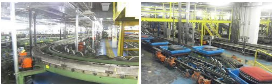
FIGURE 17: Form-fitting container conveyor system (a; b)
