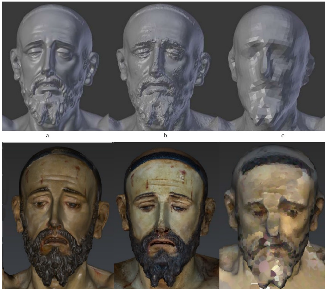
Fig. 9. Geometric detail of the faces of the 3D models of the different 3D scanning techniques. (a) Structured light scanner. (b) Photogrammetry. (c) Laser scanner.
