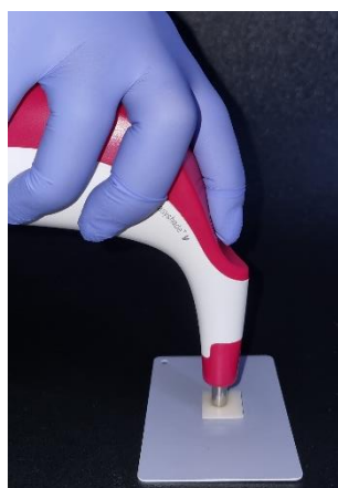
Figure 1. Colour measurement of a Telio sample on a grey background with the EasyShade V spectrophotometer.
