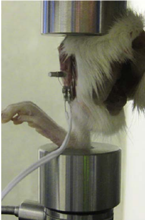
Figure 8.3 Indirect implant loading by means of compression of the implant-containing bone (tibia) through its long axis [50].
