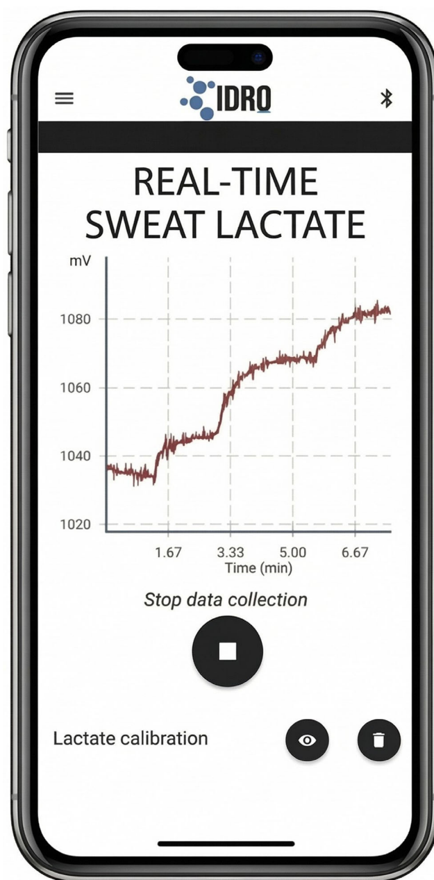
FIGURE 2 Schematic representation demonstrating real-time sweat lactate monitoring on a smartphone, showing a lactate calibration curve measured by the sensor.
