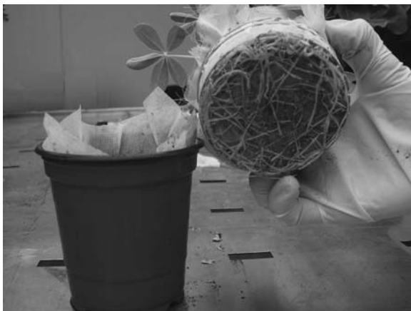
Fig. 1 The rhizopot used in the experiment. Rhizosphere soil was considered the 2-mm layer of soil placed between two nylon meshes separating the upper cylinder and the lower pot
