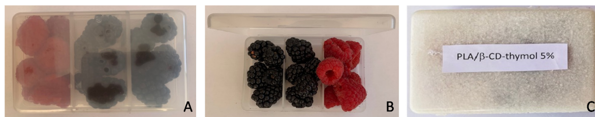
Figure 1. Boxed samples containing blackberries and raspberries. (A) PLA/C, closed; (B) PLA/β-CD-carvacrol, 2.5% wt%, open; (C) PLA/β-CD-thymol, 5.0% wt%, closed.
