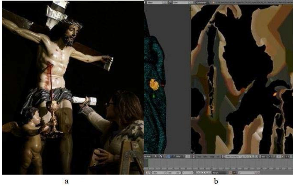
Fig. 14. (a) Sampling by spectrophotometer. (b) Identification of measurement point on the textures of the 3D models.
