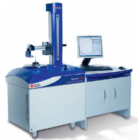
Fig. 2. Image of the apparatus used to measure the hole precision in the samples.
